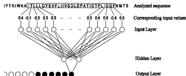
**Fig. 1.** Schematic architecture of the neural network. Amino acids of the input sequence are converted to unique input values corresponding to the propensity for each amino acid to be located inside a transmembrane region (see Table I). Output of the network consists of values between 0 and 1. Values above 0.9 (shown in black on the figure) indicate a detection of a potential transmembrane segment.
